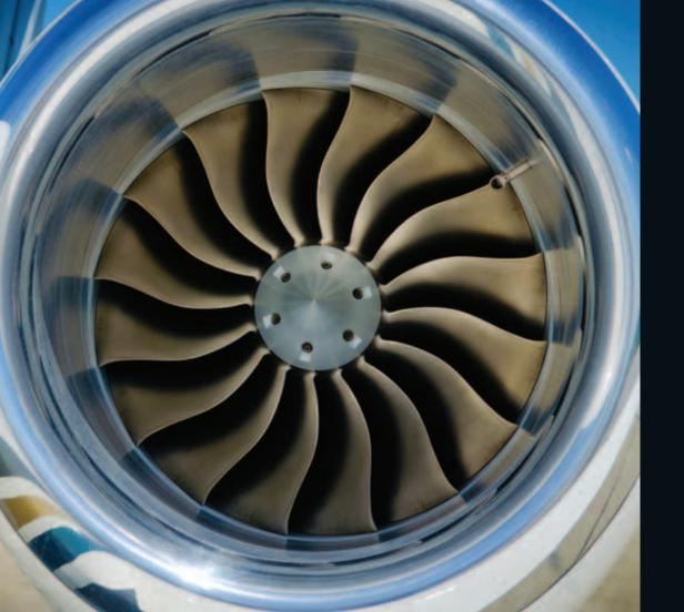
The new Williams FJ44-3AP engines are notably more fuel efficient and lighter than the original Beechjet 400A/XP Pratt & Whitney engines. As a result of the new engines, the range of the 400XT was significantly improved as well as the fuel burn.
